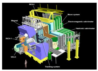
A schematic of the LHCb particle detector showing its components, one of which is the electromagnetic calorimeter.
