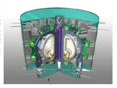
ergy. The International Thermonuclear Experimental Reactor (ITER) is a joint international research and development project seeking to build a prototype fusion power plant. (The finished machine will be located in the south of France.)
