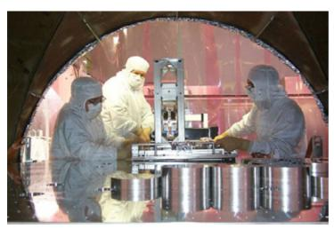
LIGO staff installing a mode-matching mirror and suspension into a vacuum chamber during the construction of LIGO. Image courtesy of LIGO
